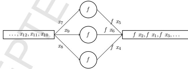
**Task farms** (*farm*) apply the same operation to each element of an input stream of tasks, using a fixed number of parallel workers. The input tasks must be independent, and the outputs can be produced in an arbitrary order.
